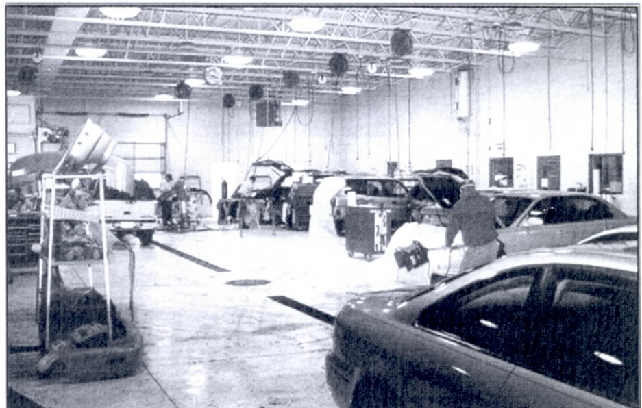
The 13,000-square-foot shop is well lit and features overhead mounted air and electrical hookups.
